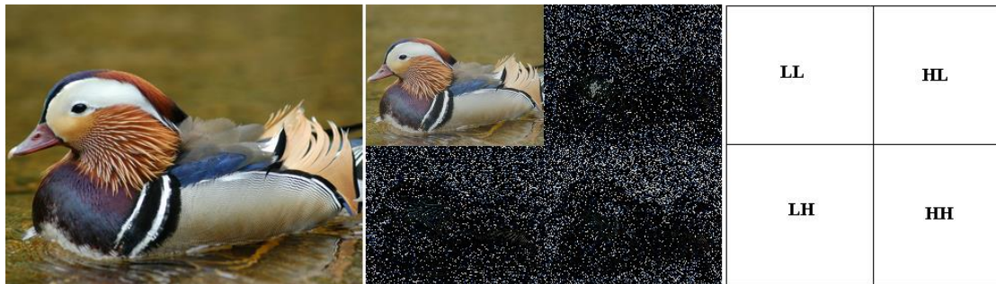
Fig. 1. The structure of the WT coefficients' grouping after the direct two-dimensional transformation of the original image
