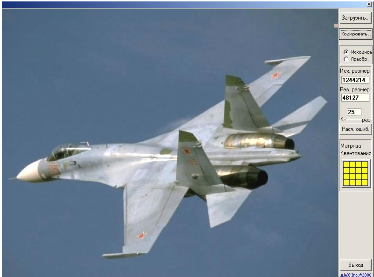
Fig. 1. The result of “the aircraft” image coding in the lossless compression mode shows a compression of 25 times, which is 48.127 kB
