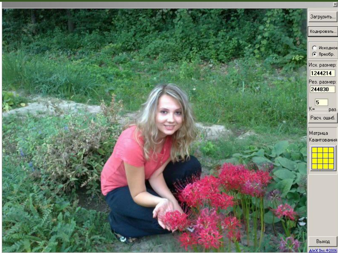
Fig. 2. The result of “the girl” image coding in the lossless compression mode shows a compression of 5 times, which is 245 KB
